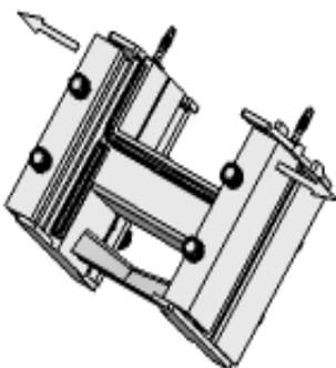
Fig. 1 Pull the sliders of the both sides
