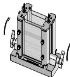
Fig. 6 Insert and tighten the cams
