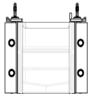
Fig. 3 Pull the sliders of the both sides
