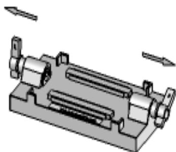
Fig. 4 Pull the cams to both sides
