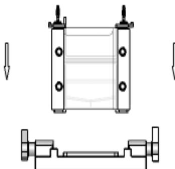
Fig. 5 Place the module in the gel cast stand
